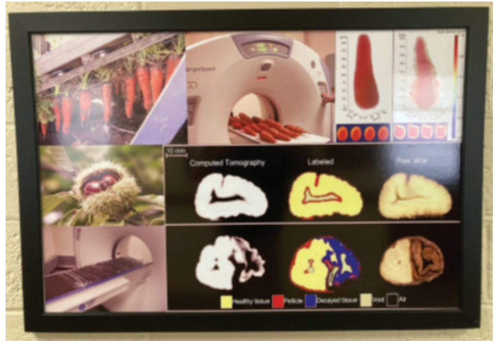
Computed tomography imaging of desirable and defective carrot and chestnut.
