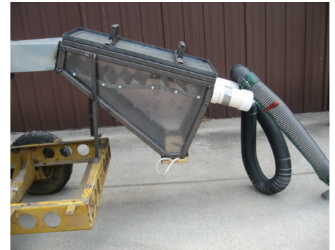
Saltation Sieve Separation concept prototype for mid-scale chestnut harvest.
